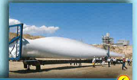
Cal Portland Cement is home to the largest behind the meter self generation wind farm in the world with eight giant 3 MW turbines, each stand nearly 400 feet tall and each blade over 140 feet long.
